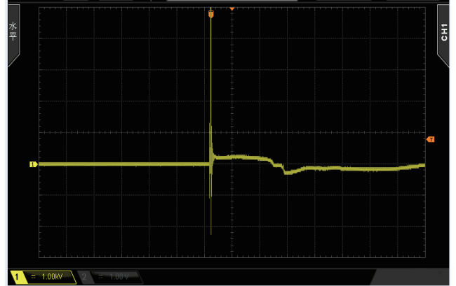
Output voltage waveform (common mode 1.3KV)
