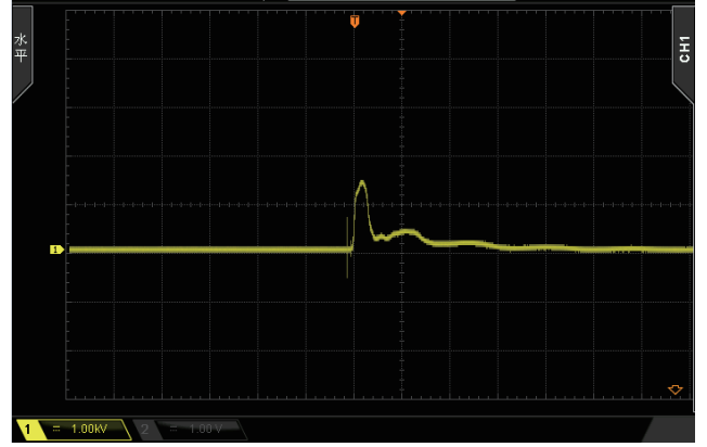
Output voltage waveform (differential mode 1.3KV)
