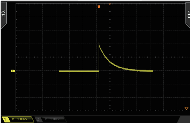
Input voltage waveform (differential mode 2KV)
